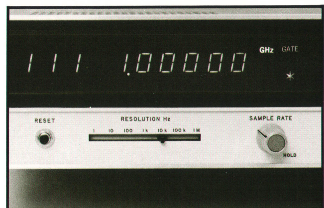
Fig. 6. An internal switch causes the counter to display the states of the two peak detectors and the frequency discriminator in the IF channel (three digits at left). These are used with the flow chart of Fig. 7 for troubleshooting.
