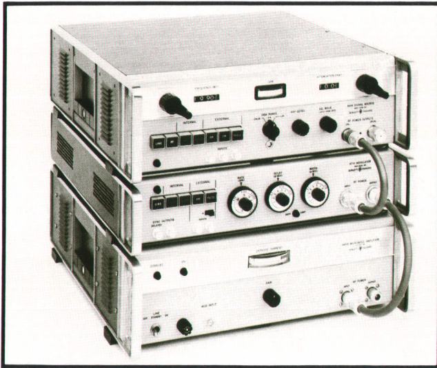
Fig. 1. System I cabinets introduced in 1961 were designed to allow the same instrument to be used either on the bench or mounted in a rack. Plastic feet fit over a cabinet below, enabling instruments to be stacked conveniently for bench use. Removal of the feet and installation of simple angle-iron brackets in the space provided enabled installation of the same instruments directly in a standard relay rack.
